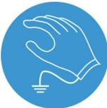
Before working on terminals on the control unit, ground yourself by touching and holding a grounded metal object (pipes, cabinets, equipment, etc.) to discharge any static electricity.
