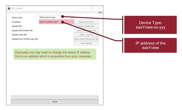
Press "Read device info" to verify that the device is successfully connected and see its status.
