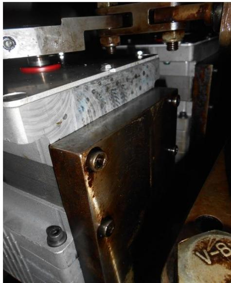
Figure 2-3. Dismantling Actuator from Mounting Plate
