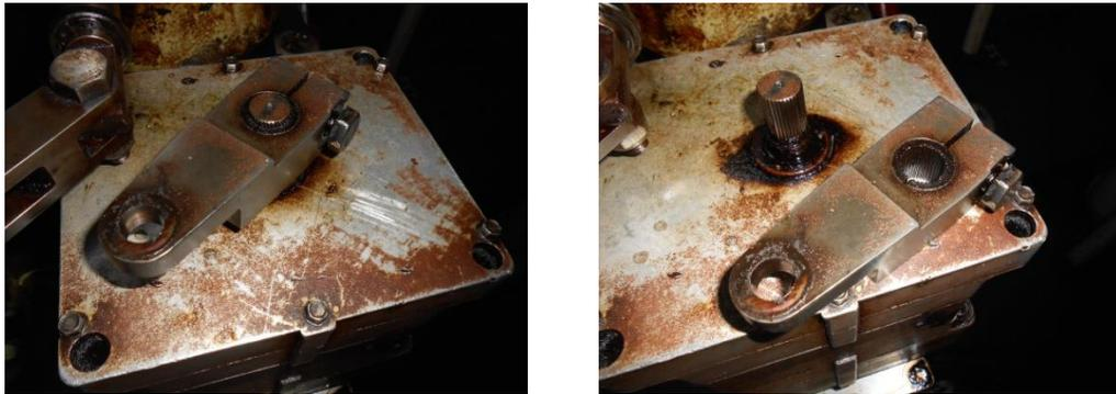
Figure 2-2. Removing Actuator Terminal Lever from Actuator Output Shaft
