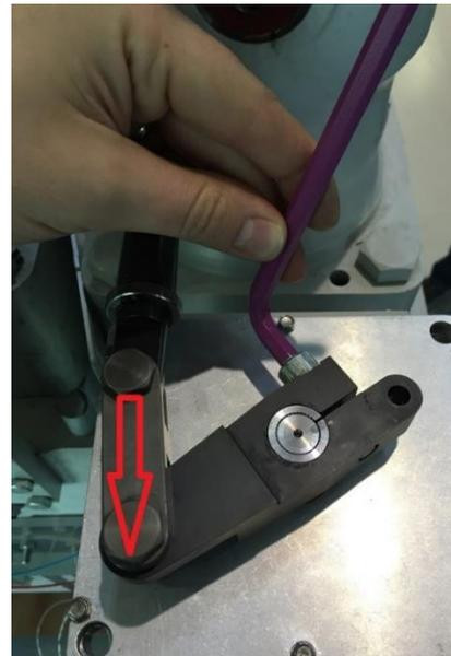
Figure 2-12. Adjusting Minimum Stop Position on the Actuator
