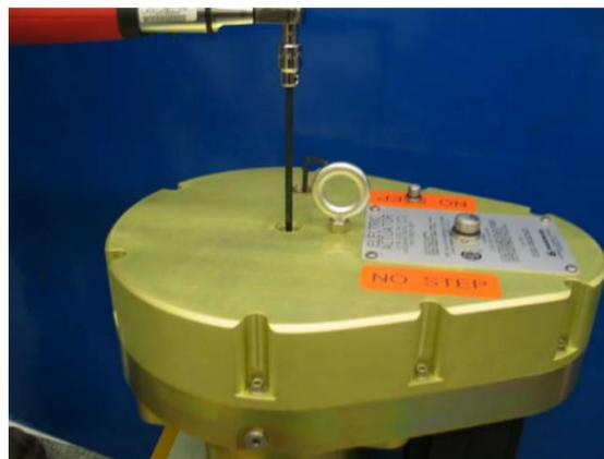
**Step L****Figure 2-4. Seating the Allen Wrench**
