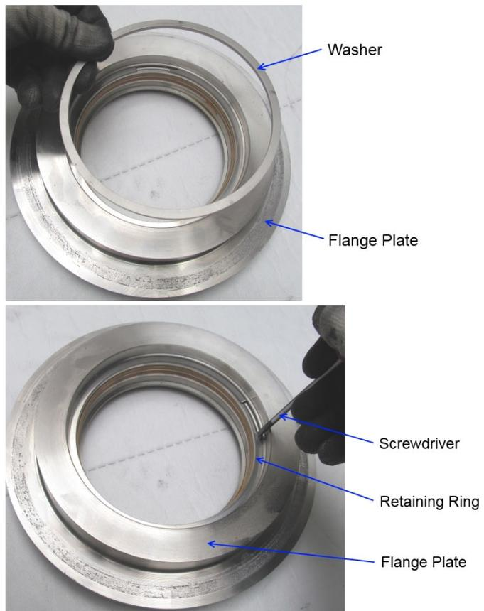
**Figure 3-3. Washer and Retaining Ring Removal**
