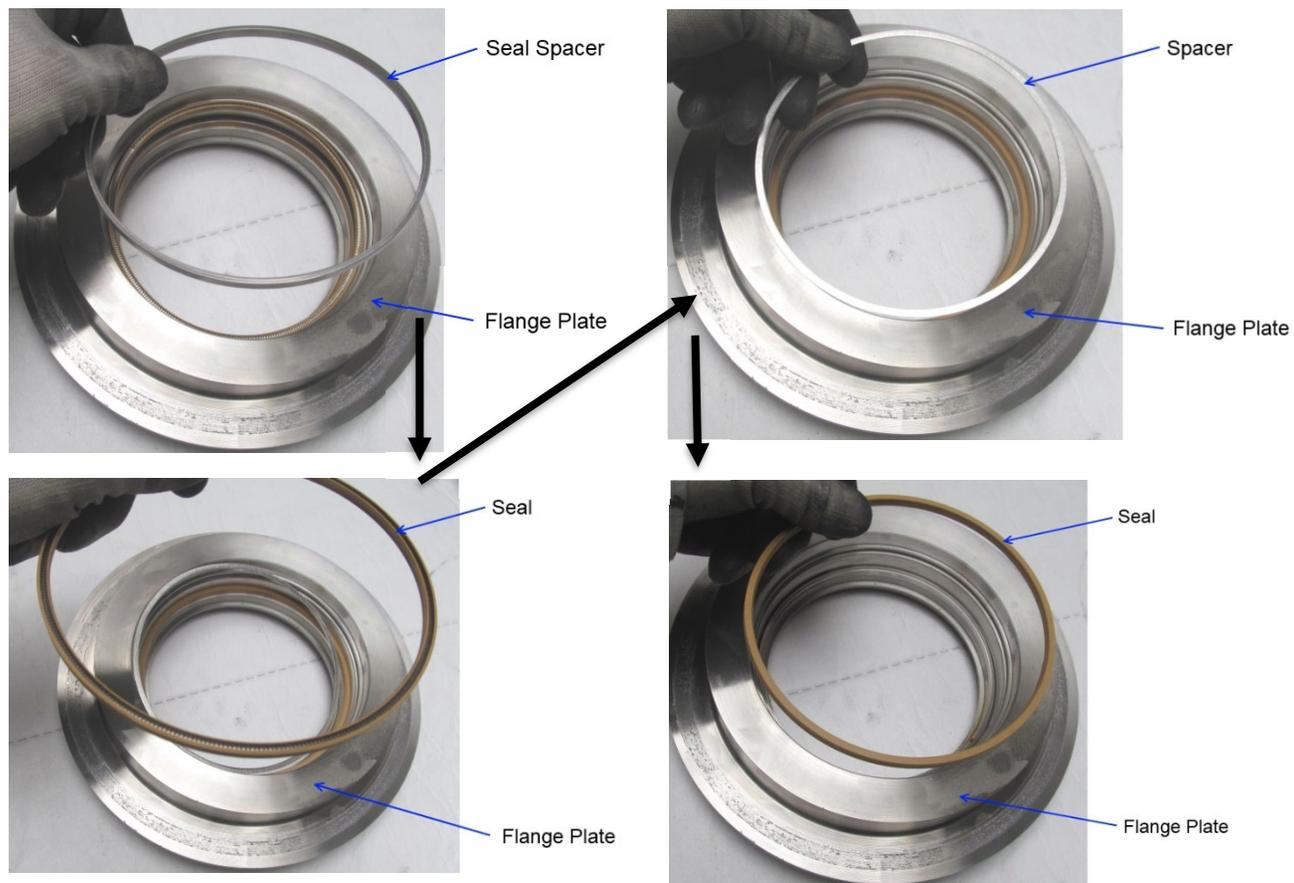
Figure 3-4. Spacer and Seal Removal
