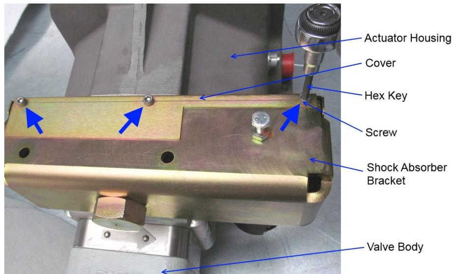
Figure 2-5. Install Cover Screws
