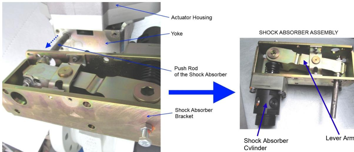
Figure 2-2. Remove Shock Absorber
