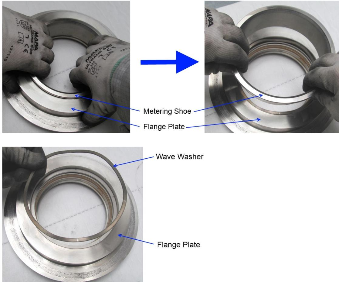
Figure 3-2. Shoe and Wave Washer Removal
