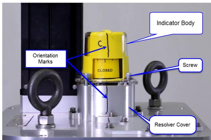
Figure 5-8. Install the Indicator Body
