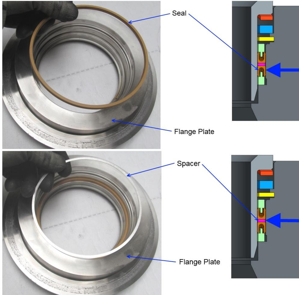
Figure 3-7. Seal and Spacer Installation
