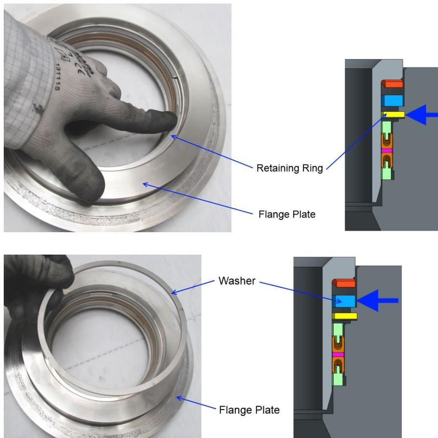
Figure 3-9. Retaining Ring and Washer Installation
