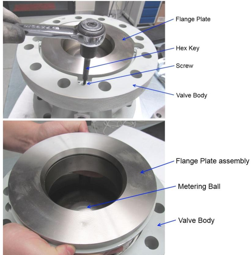
**Figure 3-1. Flange Plate Assembly Removal**
