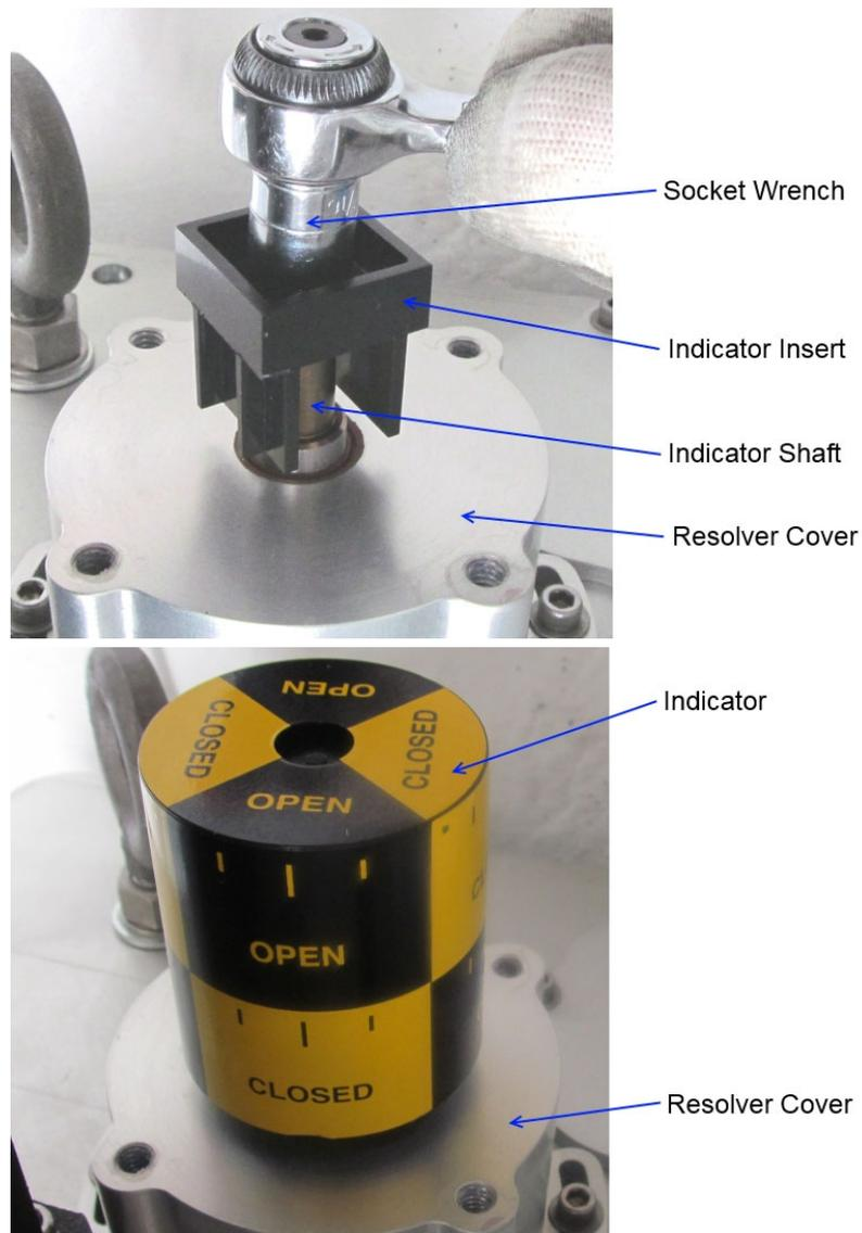
Figure 5-7. Install Indicator on the Indicator Insert
