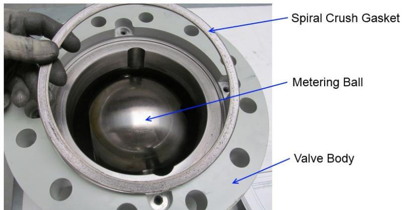
**Figure 4-5. Gasket Removal**
