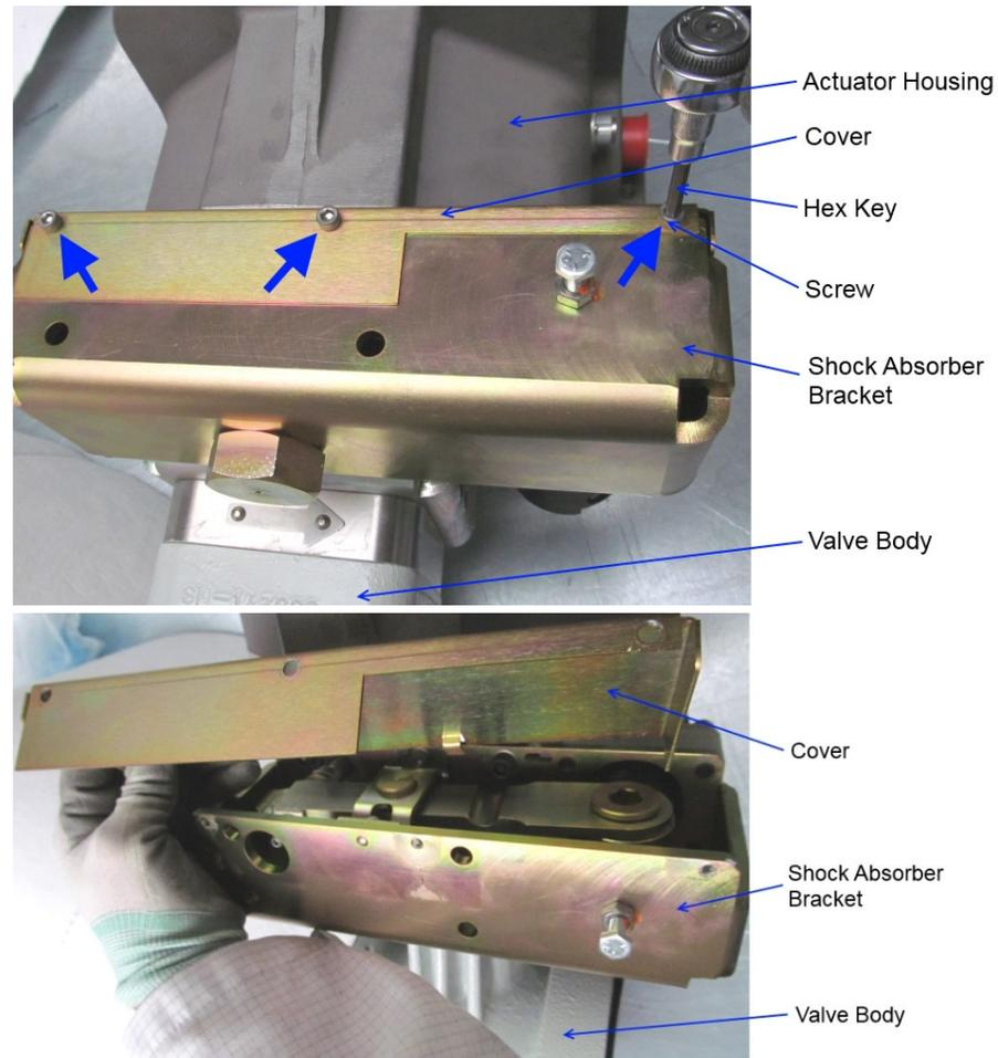
Figure 2-1. Cover and Attachment Hardware
