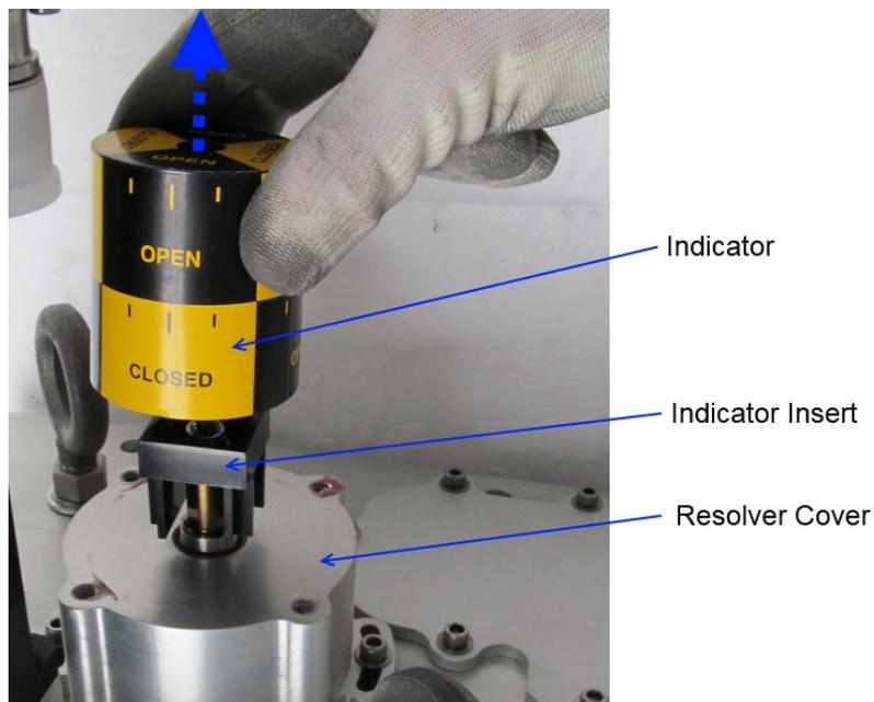
Figure 5-2. O-ring and Indicator Body Removal
