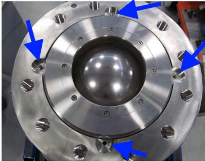
**Figure 4-1. Flange Plate Assembly Removal**
