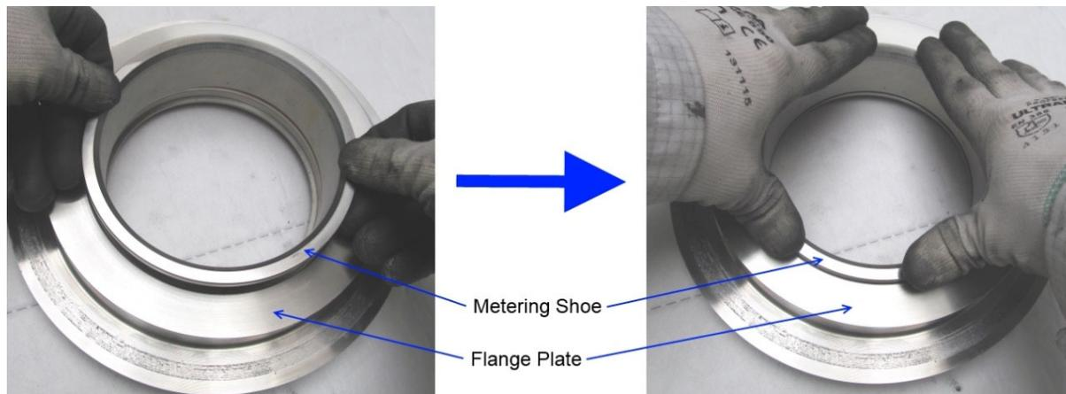
Figure 3-10. Wave Washer and Metering Shoe Installation
