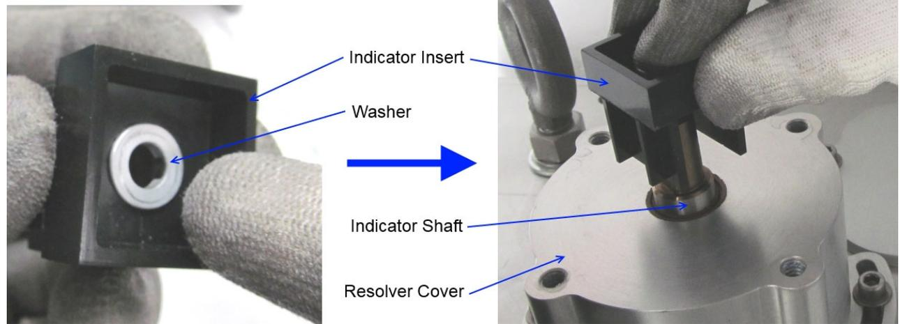
Figure 5-6. Install Indicator Insert
