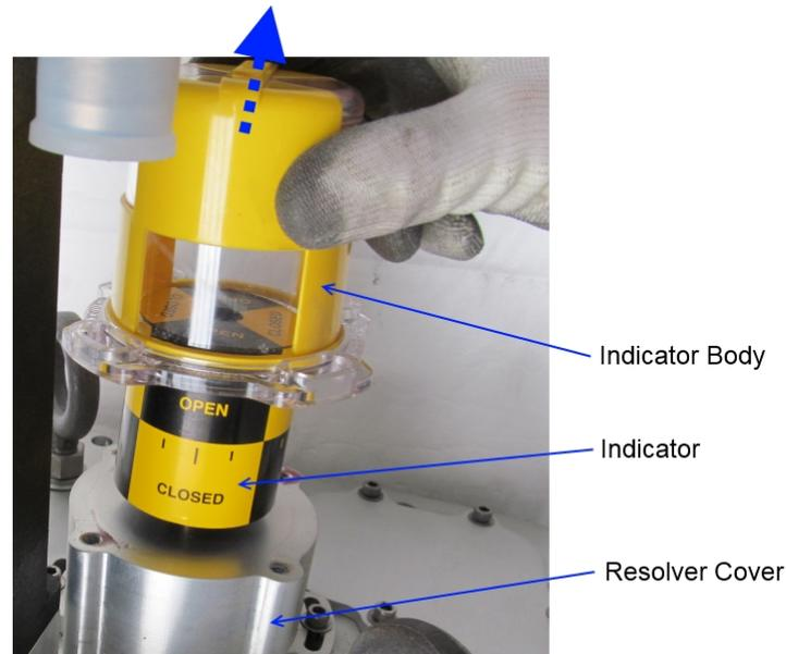
**Figure 5-1. Indicator Body Removal**
