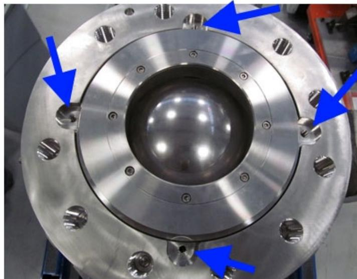
Figure 4-9. Install Gasket and Flange Plate Assembly
