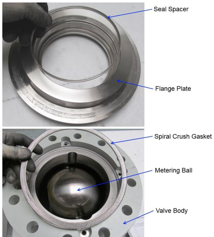
**Figure 3-5. Second Spacer Removal**
