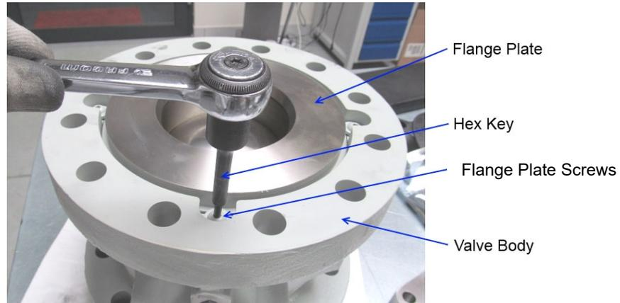
**Figure 3-12. Screw Installation**
