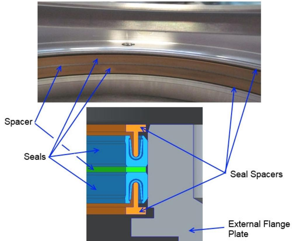
Figure 4-6. Install Seals and Spacers
