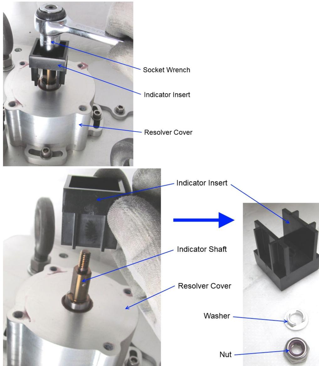
Figure 5-3. Indicator Insert Removal
