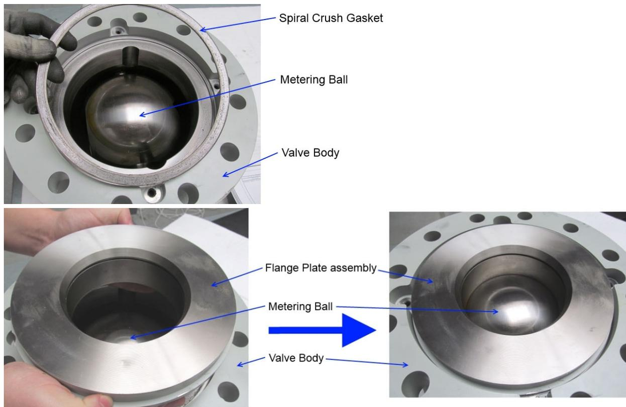
Figure 3-11. Gasket and Flange Plate Assembly Installation
