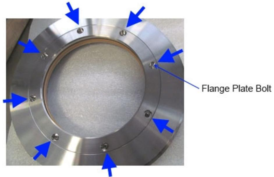
**Figure 4-3. Bolt and Flange Plate Removal**
