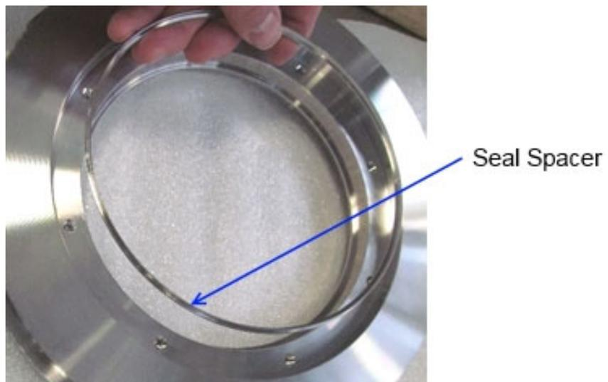
Figure 4-4. Spacer and Seal Removal
