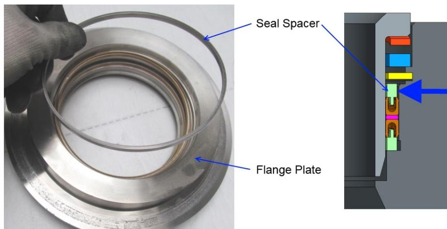
Figure 3-8. Second Seal and Spacer Installation
