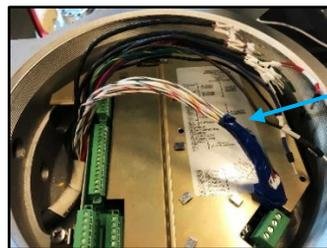
Protect wires with electrical tape
