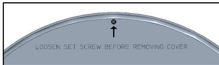
Figure 2-85. VariStroke Cover Set Screw Location
