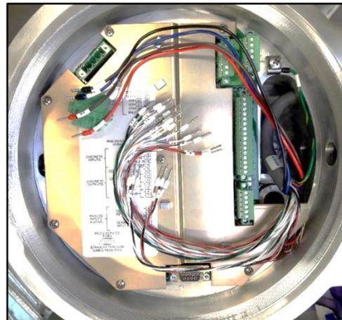
Figure 2-49. Vinyl Electrical Tape Protection Removed From Wires
