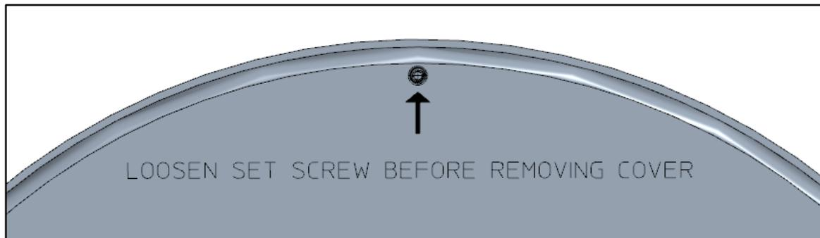
**Figure 2-27. VariStroke Cover Set Screw Installation**
