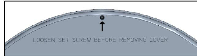
**Figure 2-6. Set Screw in VariStroke Cover**
