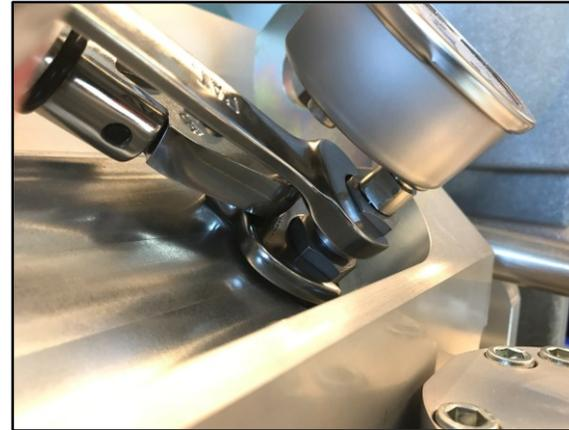
Figure 5-3. Assembling Gauge Coupling
