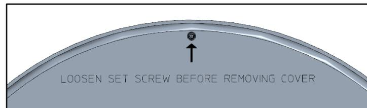
**Figure 2-43. VariStroke Cover Set Screw Location**
