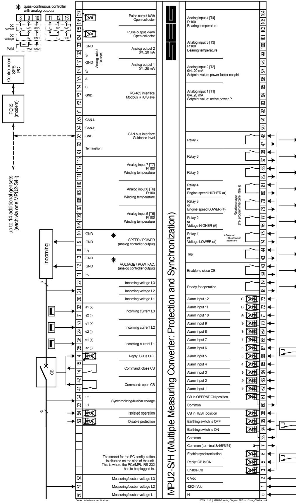
MPU2-S/H (Multiple Measuring Converter: Protection and Synchronization)
