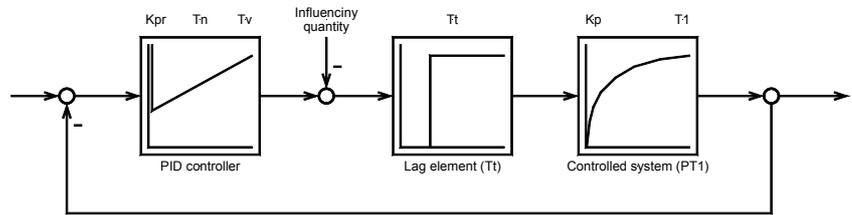
If an abrupt disturbance variable is applied to the control loop, the reaction of the controlled system can be recorded at the output as a function of time (step response).
