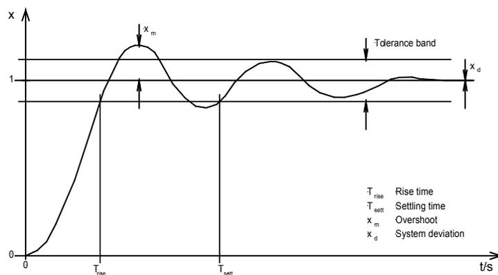
Various values can be obtained from the step response; these are required for adjusting the controller to its optimum setting:
