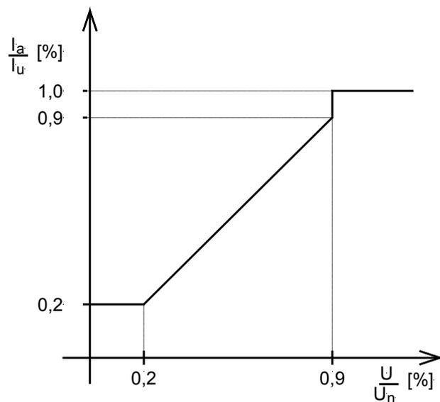
Data meaning:  $I_a$  = adjusted threshold,  $I_u$  = setting value,
