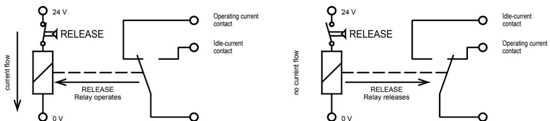
Example Digital inputs 1 through 4 (same procedure for inputs 5-12)
