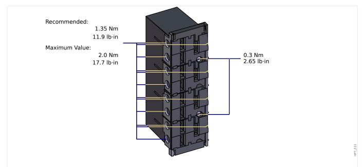
Fig. 137: Plug-in Connector with Integrated Short-Circuiter (Conventional Current Inputs)
