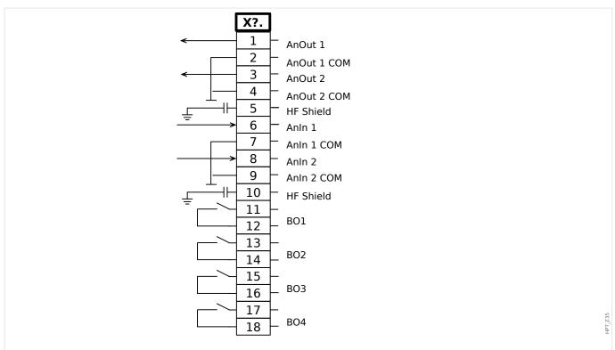
Fig. 38: Terminal Marking.
