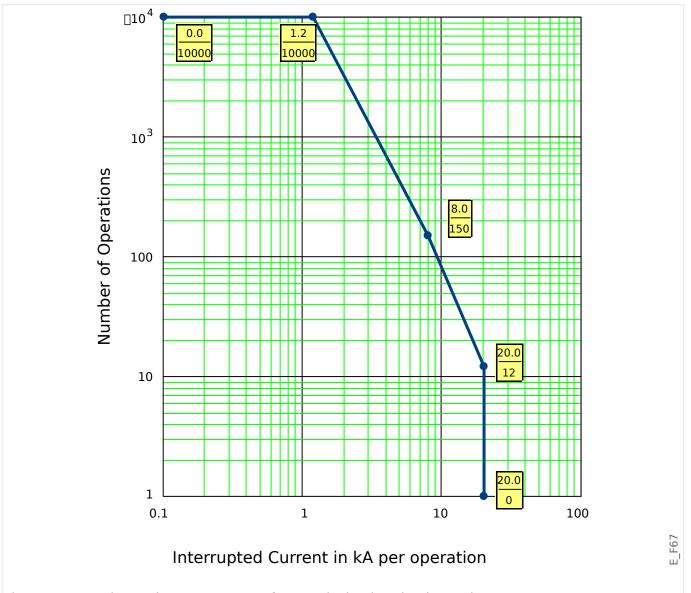
Fig. 124: Breaker Maintenance Curve for a typical 25kV Circuit Breaker
