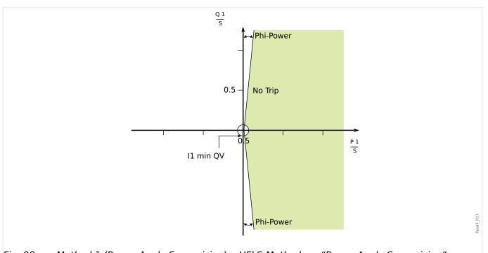
Fig. 99: Method 1 (Power Angle Supervision): »UFLS-Method« = "Power Angle Supervision".
