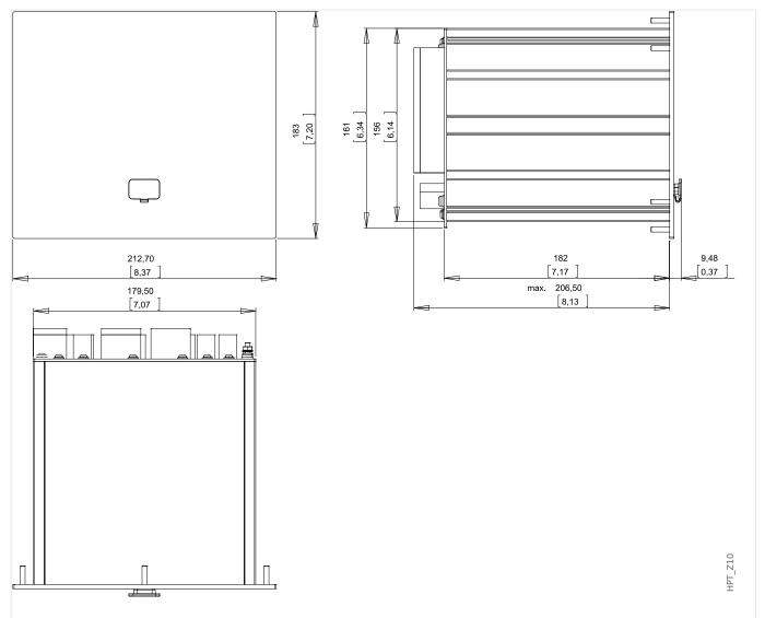
Fig. 5: 3-Side-View B2 Housing (Devices with 8 Softkeys). (All dimensions in mm, except dimensions in brackets [inch].)
