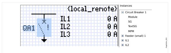
Fig. 118: Control Page Example, with the "Circuit Breaker" being highlighted.
