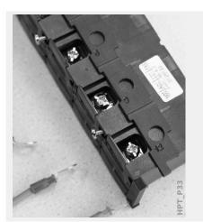
Move the slider aside, so that the screws and metal contact become fully accessible.
