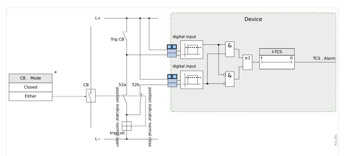
Fig. 115: Connection example: Trip circuit supervision with two CB auxiliary contacts »Aux ON« (52a) and »Aux OFF« (52b).
