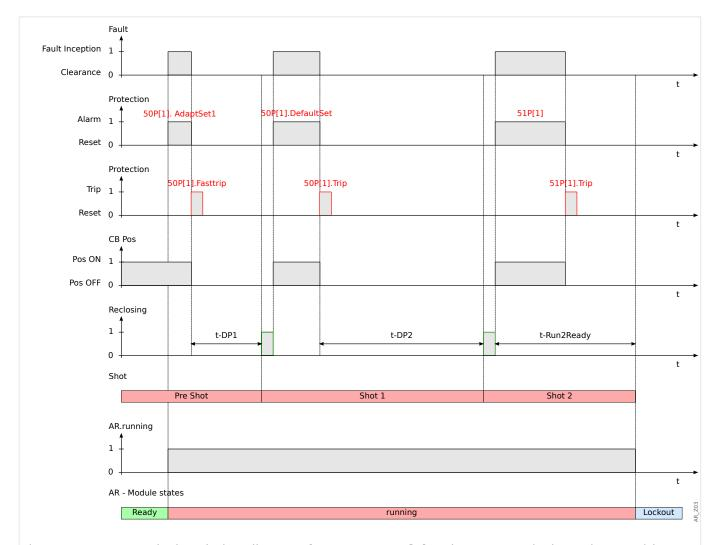
Fig. 103: Auto Reclosing timing diagram for **unsuccessful** 2-shot auto reclosing scheme with acceleration at pre-shot.
