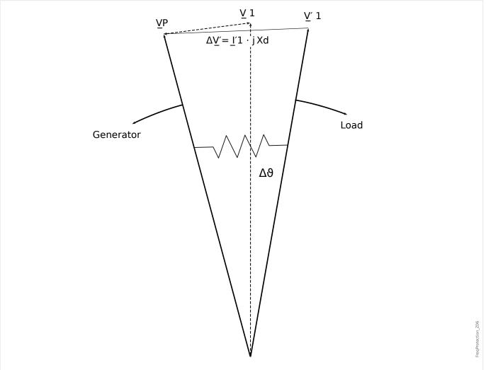
Fig. 87: Voltage vectors at mains failure.
