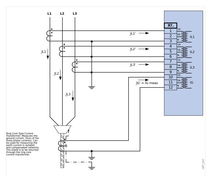
Fig. 20: Three phase current measurement; In secondary = 1 A. Earth-current measuring via cable-type current transformer; IGnom secondary = 1 A.
