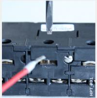
For the pin-terminal connection type, insert the cables and fasten them by the screws that are located at the side of the input card.
