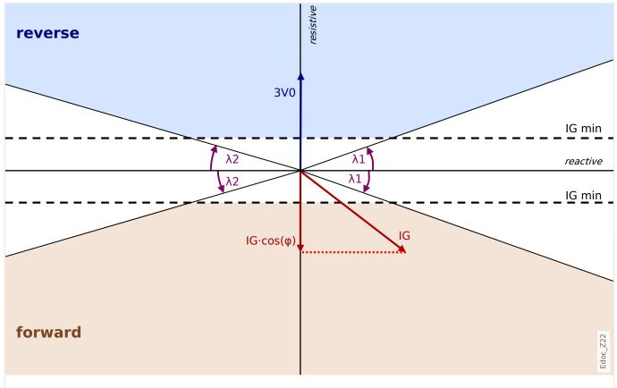
Fig. 66: Principle of direction determination for the method " $cos(\phi)$ ".
