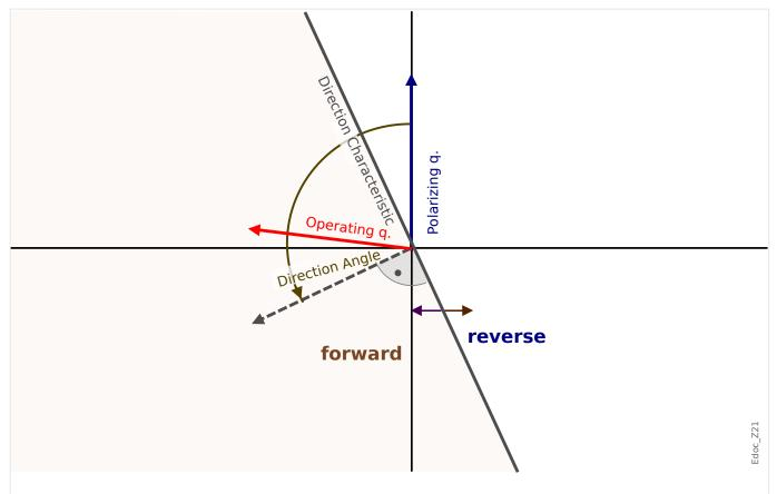
Fig. 64: Principle of direction determination for all methods except " $cos(\phi)$ ", " $sin(\phi)$ ".
