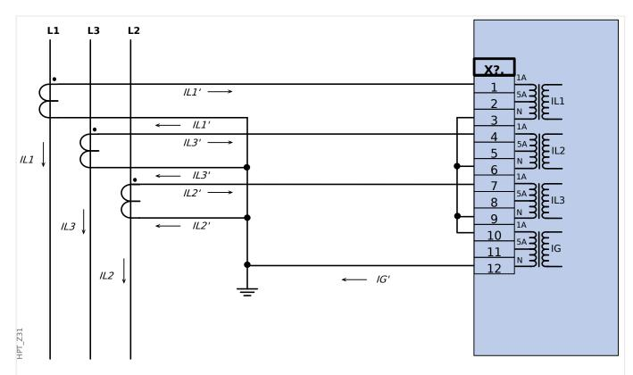
Fig. 24: Three phase current measurement; In secondary = 1 A. Earth-current measuring via Holmgreen-connection; IGnom secondary = 1 A.
