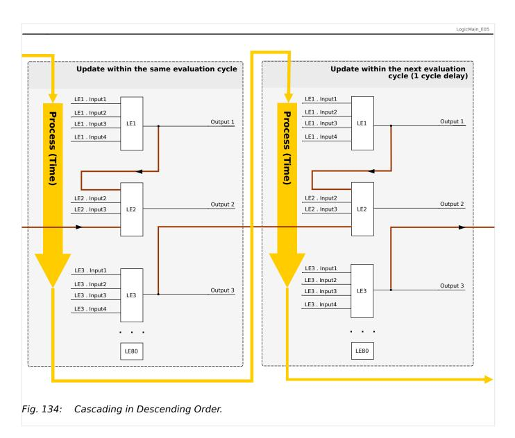
In the example shown in  $\sqsubseteq$  Fig. 134 above, "Logic Equation 2" uses the output states of two other equations, "Logic Equation 1" and "Logic Equation 3". The result of "Logic Equation 1" is used in ascending order and has therefore been evaluated within the same process cycle. The result of "Logic Equation 3" is used in descending order and has therefore been evaluated in the previous process cycle.
