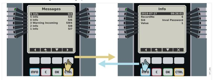
Fig. 136: Example display of the Self-Supervision messages.
