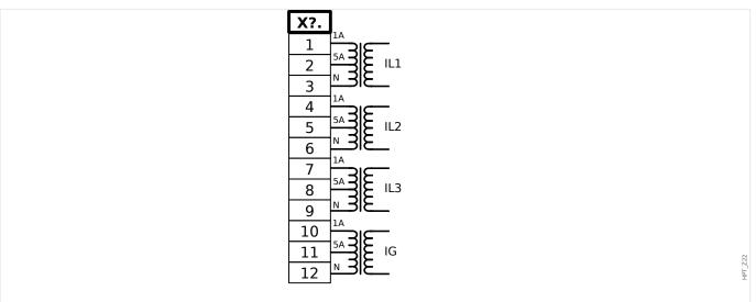
Fig. 15: TI - Terminal Marking
