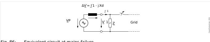
Fig. 86: Equivalent circuit at mains failure.
