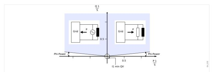
Fig. 91: Method 1: Power Angle Supervision.
