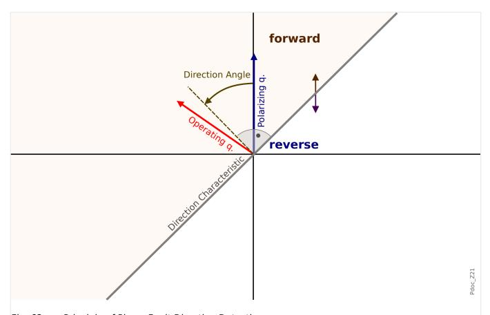
Fig. 62: Principle of Phase Fault Direction Detection.
