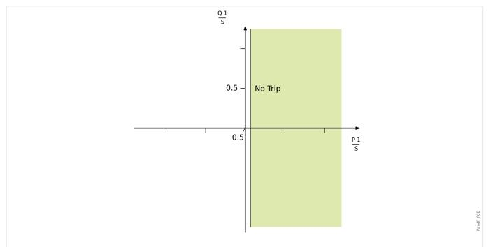
Fig. 100: Method 2 (Pure Active Power Supervision): »UFLS-Method« = "Pure Active Power Superv".
