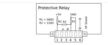
Fig. 46: Electro-mechanical assignment
