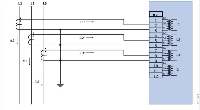
Fig. 19: Three phase current measurement; In secondary = 5 A.
