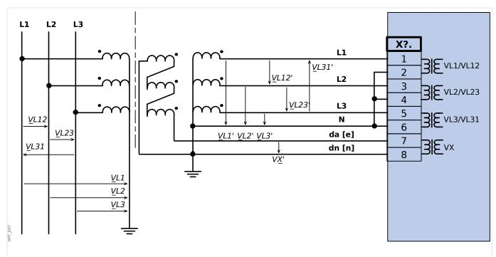
Fig. 31: VT Wye with Broken Delta Connection.
