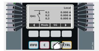
By pressing the »CTRL« key you enter a screen showing the single line, and you have direct access to related measuring values and control functions.
