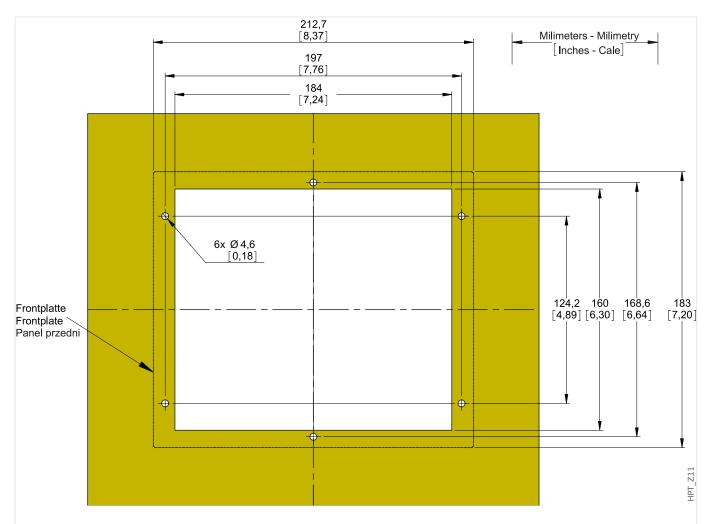
Fig. 6: B2 Housing Door Cut-out (8 Pushbutton Version). (All dimensions in mm, except dimensions in brackets [inch].)
