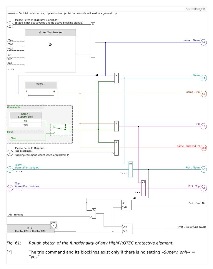
This diagram shows the basic idea behind a protective element. (Nevertheless, keep in mind that device-specific or protection-specific deviations are possible: Some devices do not feature voltage measurement, other do not feature current measurement, for some
