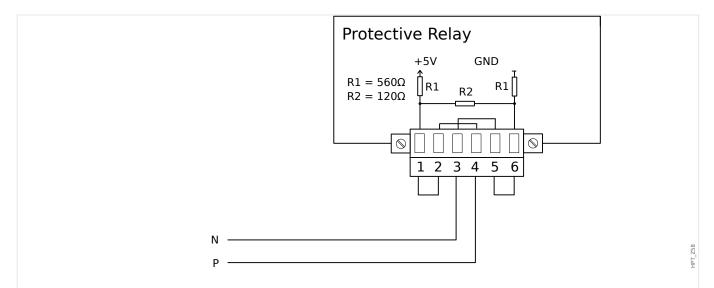
Wiring example, Device at the end of the bus. (Setting wire jumpers to activate the Fig. 48: integrated Terminal Resistor.)
