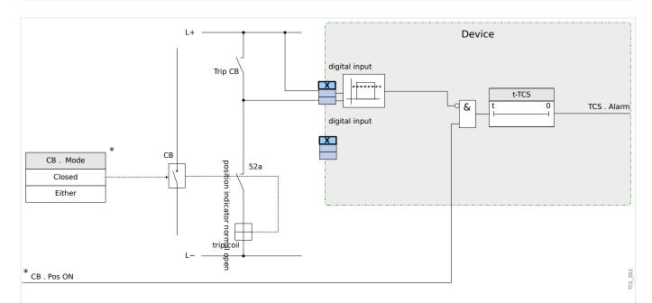
Fig. 116: Connection example: Trip circuit supervision with only one CB auxiliary contact »Aux ON« (52a).
