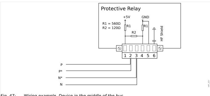
Fig. 47: Wiring example, Device in the middle of the bus
