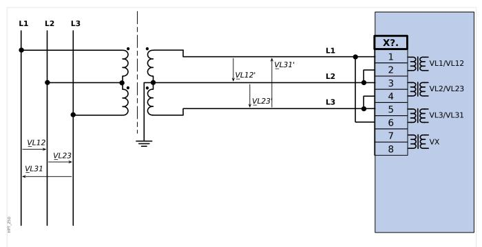
Fig. 34: Two-phase voltage measurement - wiring of the measuring inputs: "Open Delta"
