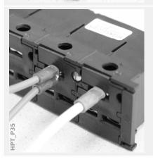
Remark: As long as the cable cross-sections are within the limits given in the Technical Data chapter ( "12 Technical Data", Tab. ) it is also possible to insert two rings into one terminal, as shown here. This is useful for setting up the neutral point connection.
