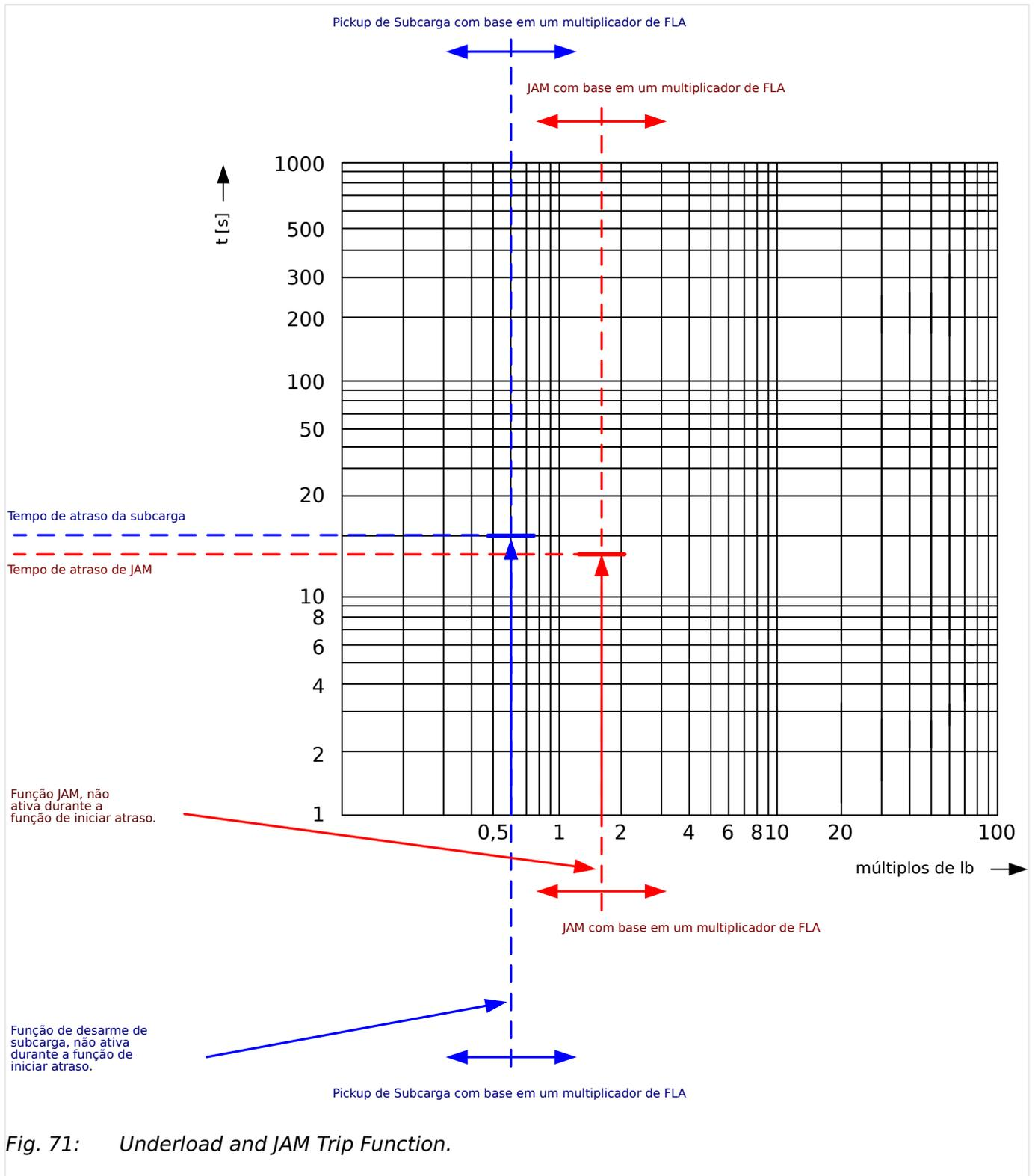
Fig. 71: Underload and JAM Trip Function.
