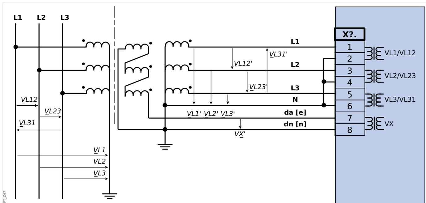
Fig. 29: VT Wye com conexão Broken Delt.
