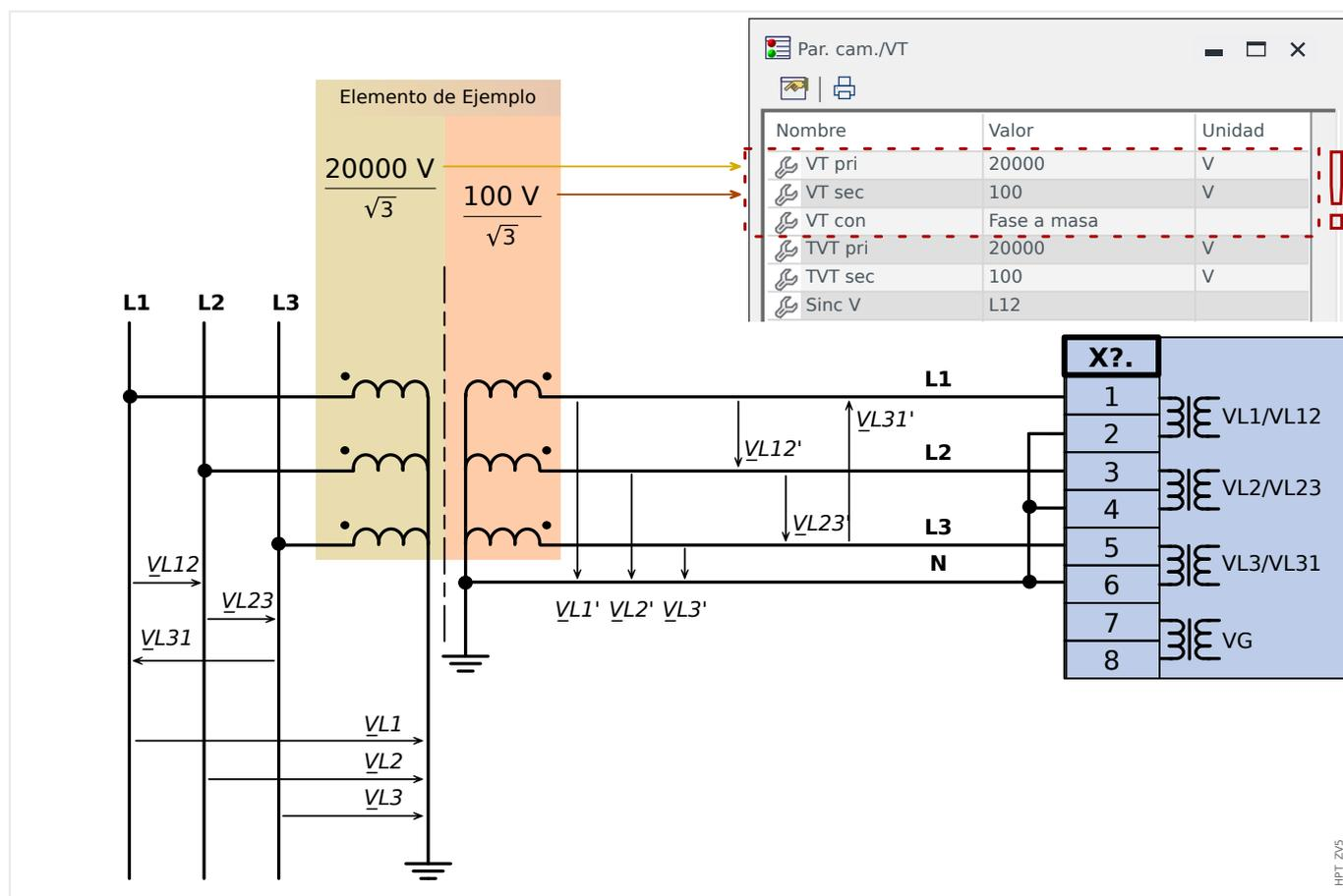
The residual voltage is calculated from the three phase-to-ground voltages with the following setting:
